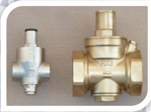
Inlet outlet 1/4 3/8, 1/2, 3/4, 1, 1 1/2 inch. Adjustable from 2 bar to 8 bar Operating pressure 2 bar to 16 bar Has a 1/4 inlet for a pressure gauge to monitor pressure. (Gauge can be left in place or removed once regulator has been set)
